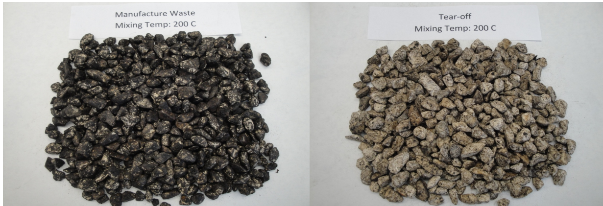
Figure 8. RAS Binder Transfer to Limestone Aggregates at Four Different Temperatures.
